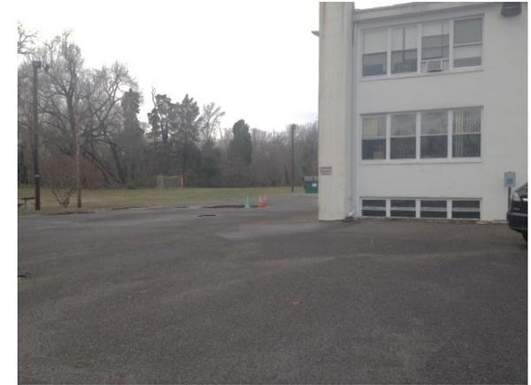
Stormwater is currently directed to the parking lot which connects to one storm drain on the property. Parking spots by the west and south side of the building can be replaced with pervious pavement to capture and infiltrate stormwater. Downspout planter boxes can be installed in the front of the building to capture rooftop runoff. A preliminary soil assessment suggests that the soils have suitable drainage characteristics for green infrastructure.
