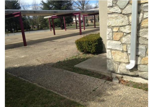
Sections of the courtyard can be replaced with pervious pavement to intercept and infiltrate stormwater. A preliminary soil assessment suggests that the soils have suitable drainage characteristics for green infrastructure.
